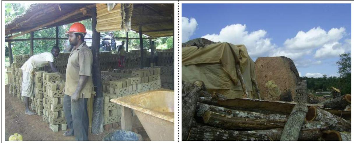
Plate 3. An example of logs used by artisanal brick makers
